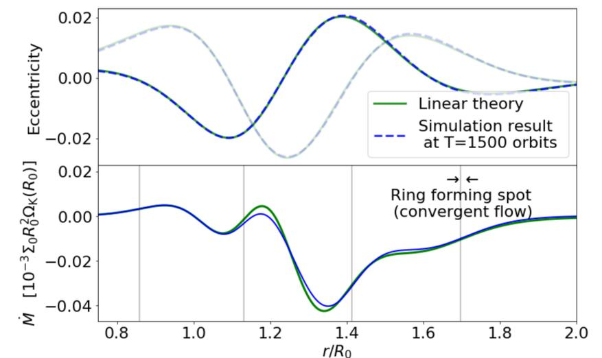
**Figure 4.** Comparison between the linear theory prediction and hydro simulation results at  $T = 1500$  orbits:
